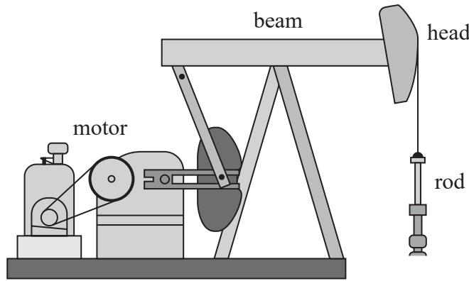
The motor raises and lowers one end of the beam, causing the head of the beam to move with simple harmonic motion. The head is attached to a metal rod that moves up and down, operating a pump deep in an oil well.
